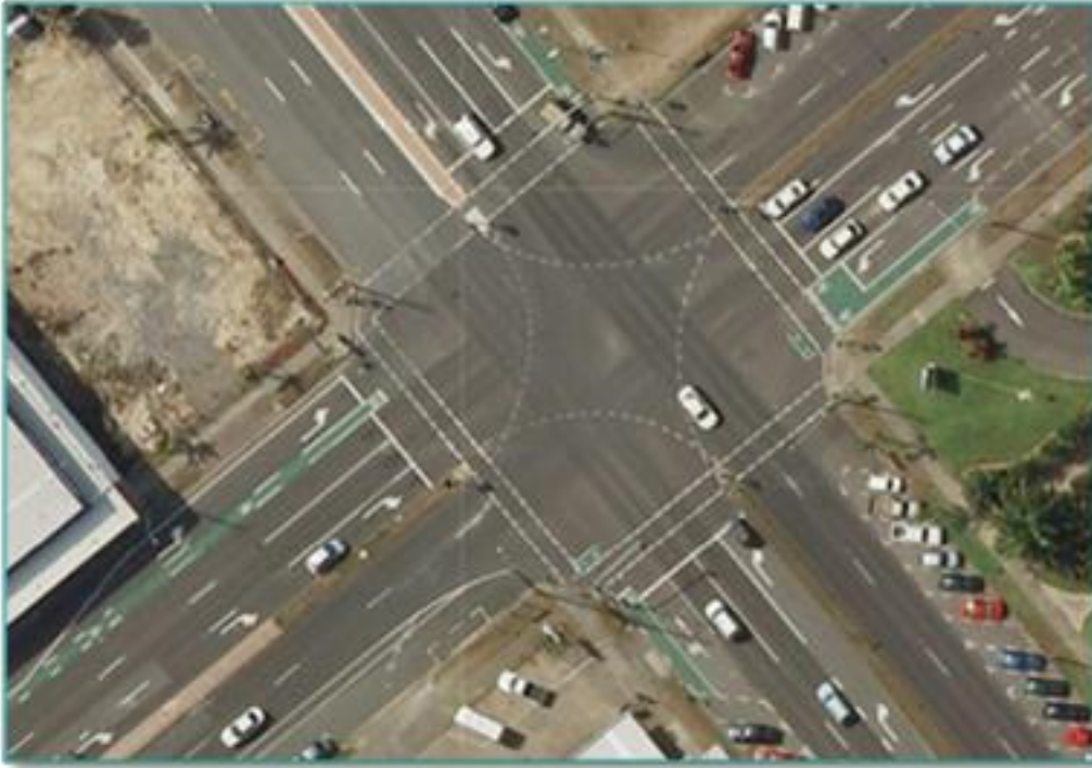
Figure 26 Expanded storage and hook turn at signalised intersection
